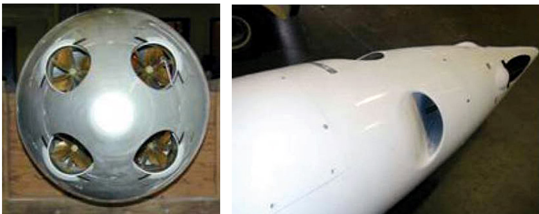
Figure 59. Distributed multi jets propulsor inlets (right) and outlets (left).
