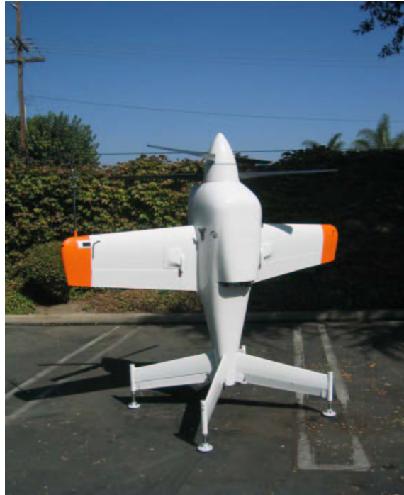
Figure 56. Skytote counter rotating vertical-landing UAV. Source: AeroVironment.
