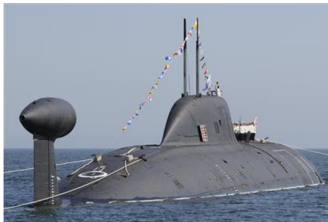
Figure 46. Akula Class Russian nuclear submarine with its tail sonar gear.
