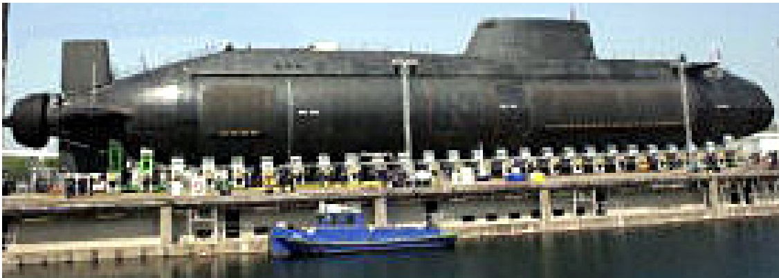
Figure 61. HMS Astute class of attack submarine on rollout showing the lampshade noise suppression duct surrounding its shrouded jet propulsor. Source: BAE Systems, UK.
