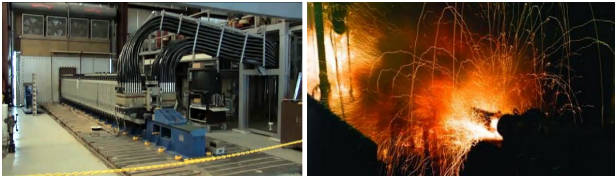
Figure 58. Railgun experimental setup and firing.
