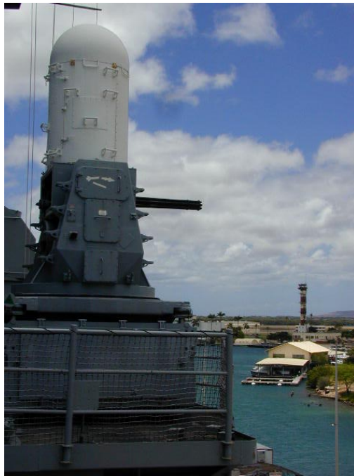
Figure 22. The Phalanx radar-guided gun, nicknamed as R2-D2 from the Star-Wars movies, is used for close-in ship defense. The radar controlled Gatling gun turret shooting tungsten armor-piercing, explosive, or possibly depleted uranium munitions on the USS Missouri, Pearl Harbor, Hawaii. Photo: M. Ragheb.
