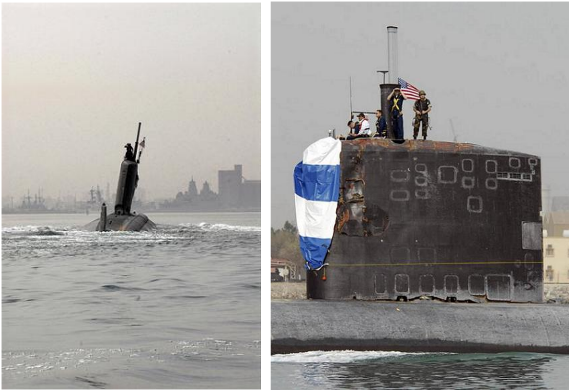
Figure 48. The collision of the Hartford with the New Orleans on March 20, 2009 caused damage to its communication gear and bent its sail.
