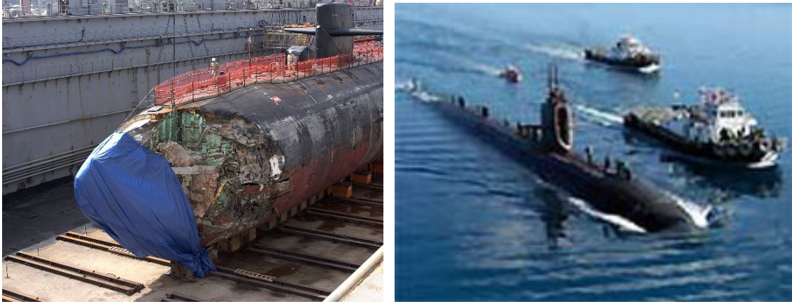
Figure 45. Location of sonar dome on the Astute class of submarines, UK. USS San Francisco SSN 711 accident, January 8, 2005. Damage from the glancing collision to the bow dome and to the double hull structure can be observed. A bulge over the hull can also be noticed.
