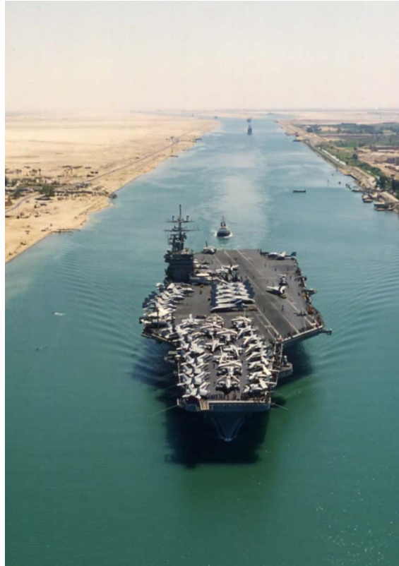
Figure 1. Nuclear aircraft carrier USS Theodore Roosevelt, Nimitz Class CVN-71, powered with two A4W (A for Aircraft carrier, 4 for fourth generation and W for Westinghouse) nuclear reactors with 100 MW of power each, crossing the Suez Canal, Egypt, during the first Gulf War, January 1991. Source: USA Navy.
