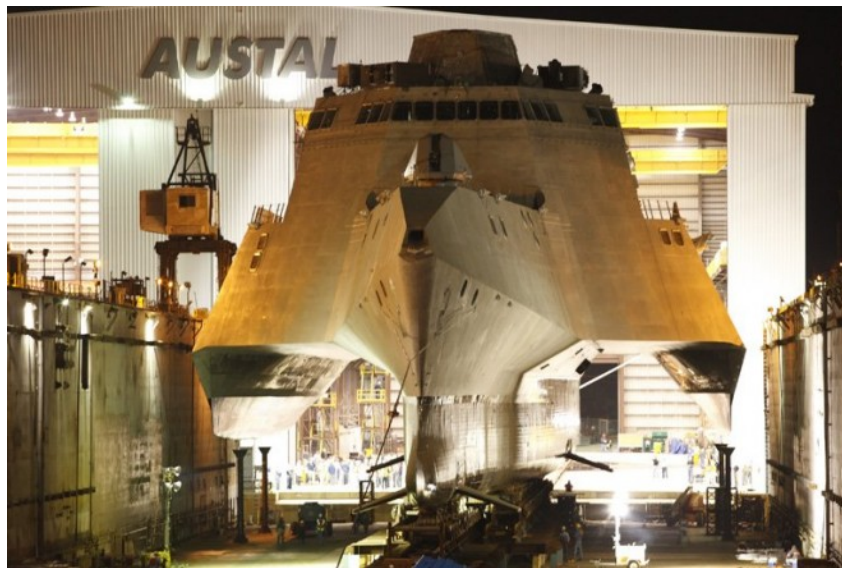
Figure 57. Trimaran Littoral Combat Ship uses water jets propulsion. Source: Austal.
