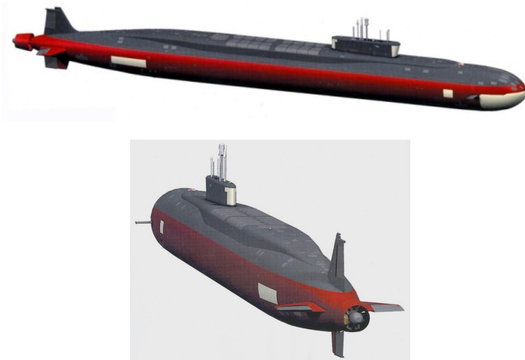
Figure 62. Lampshade noise suppression system surrounds the jet pump propulsor in the Moray class submarine, Canada. Source: United NW Canada.
