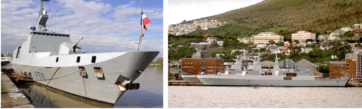
Figure 51. Stealth radar deflecting technology implemented into a French Lafayette class frigate, 2001 (left). The South African stealth Valour class frigates, built by Blohm + Voss from Hamburg, Germany to the MEKO A-200SAN design, uses both screws and water jets, in a “Waterjet and Refined Propeller” or WARP arrangement, with three shaft lines. A single GE LM2500 gas turbine and a pair of MTU 16V1163 TB93 diesels drive Lips controllable-pitch propellers outboard and a single Lips LJ2 10E water jet on the centerline.
